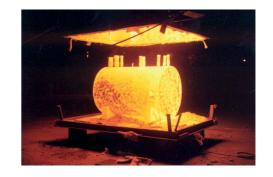
"THE SUPERVAULT'S UNIQUE PERFORMANCE SPECIFICATION OF A FOUR-HOUR FIRE RATING TOGETHER WITH ITS MULTI HAZARD ACCREDITATION, PUTS IT AT THE FOREFRONT OF TANK SAFETY TECHNOLOGY"
